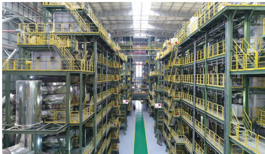
**Two continuous galvanizing lines implemented at Baotou Iron & Steel Group in China**
