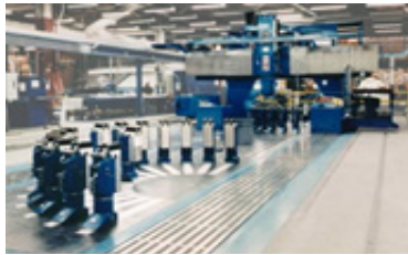
"Heavy" curved chord tooling with specific prehension
