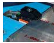
Unilateral automatic clamping system to reduce loading/unloading time
