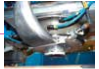
Pressure bowl and optimized chip vacuum system to increase part quality
