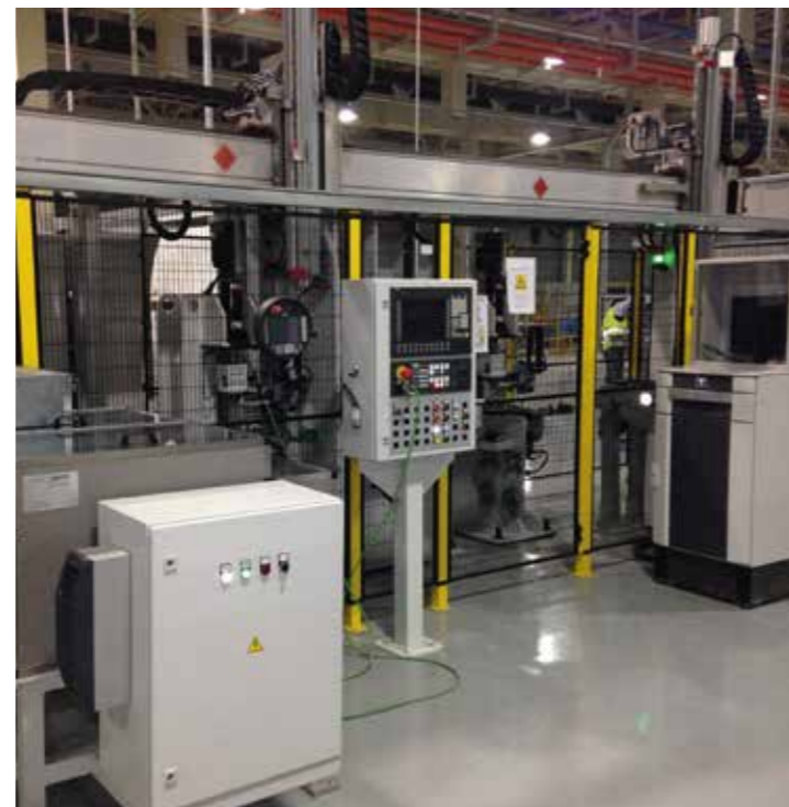
Automated laser welding line for automatic transmission gearset
