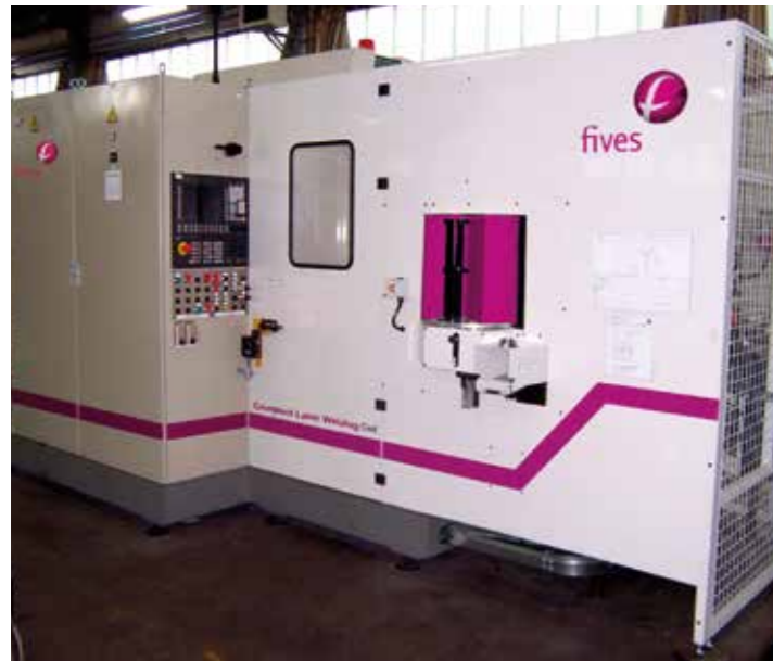
Laser welding machine for speed gears
