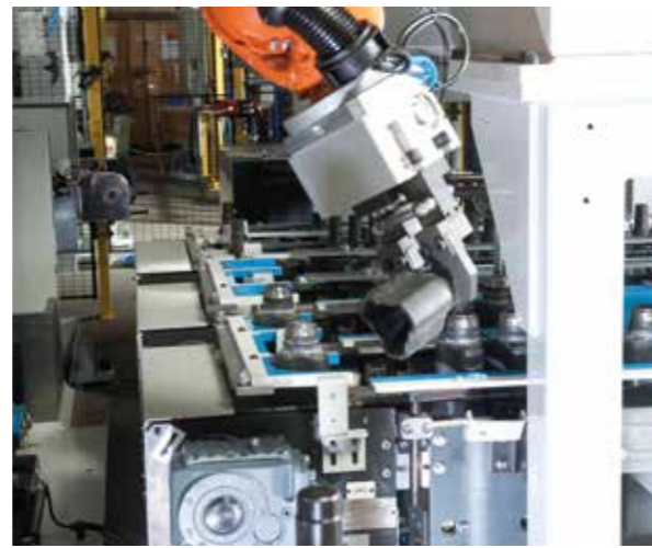
Laser welding cell for transmission shafts
