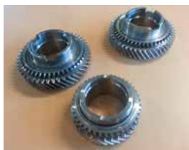
Laser welded components of Manual Transmission gearset, Dual Clutch Transmission
