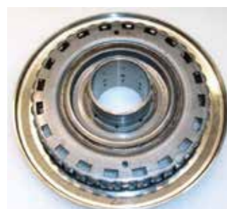
Laser welded components of Manual Transmission gearset, Dual Clutch Transmission
