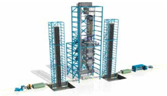
Combining Fives Celes' transverse flux induction technology EcoTransFlux™ with Fives Stein's FlashCooling rapid cooling technology, the iBAL systems allows the annual processing of as much as 350,000 tonnes of bright annealing stainless strips of BA quality.
