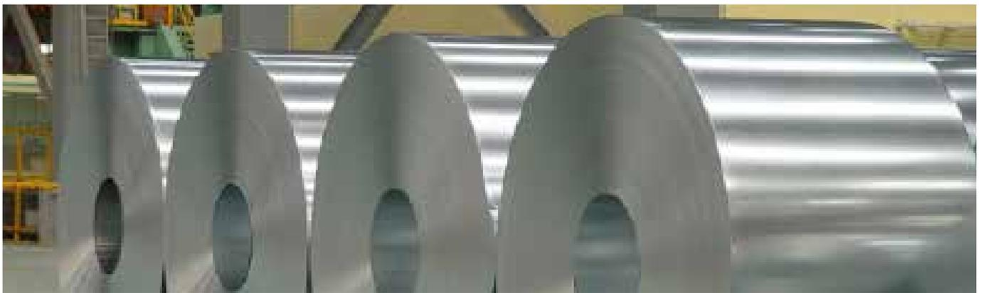
Cold rolled steel after continuous Annealed process
