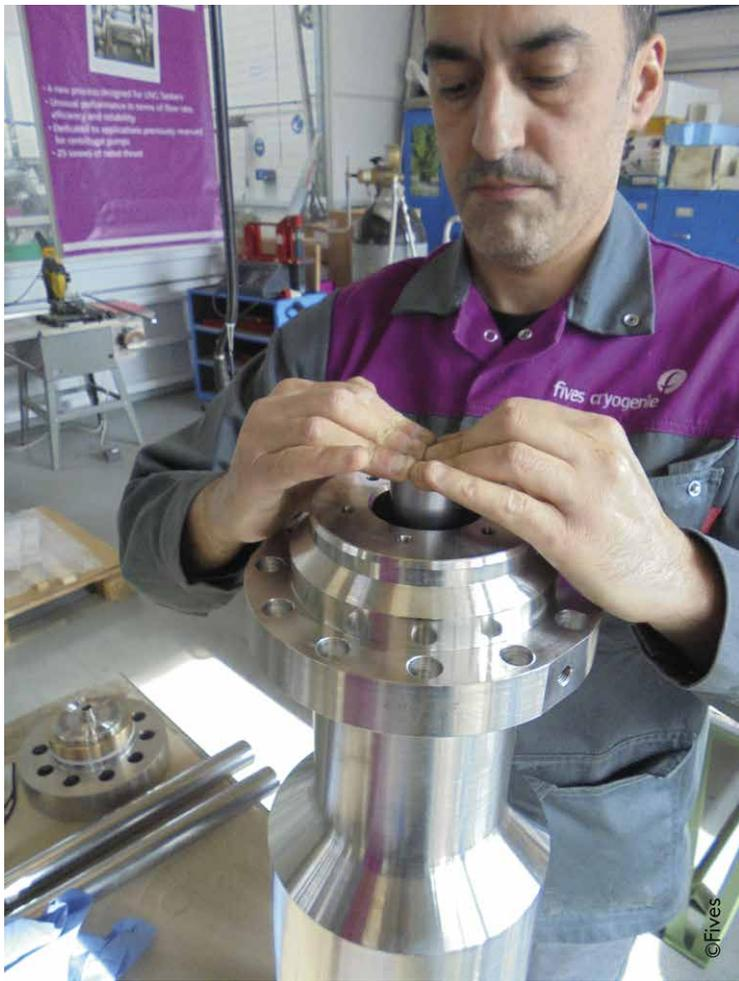
**Figure 5 - Piston head maintenance for a FGSS piston pump**
