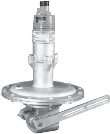
Valve positioners employ the full force of their air supply to drive the piston or diaphragm in a pneumatic actuator to the position called for by a control instrument—and to hold that position, regardless of the forces which tend to change valve position.
