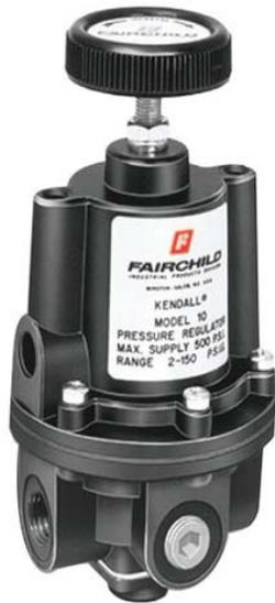
The R690-1407 Compressed Air Pressure Regulator is recommended for use with the 7266-0 Multiplying Air Regulator to insure a constant air supply pressure. Install the R690-1407 upstream of the 7266-0, and also upstream of the 8645A-01 Air Filter-Separator if one is used.
