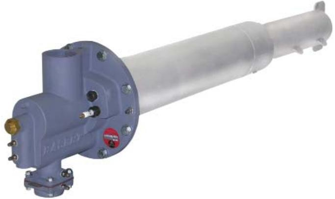
The 4748 RASERT has a number of advantages over conventional SERT's. Since the flame is in direct contact with the inside surface of the radiant tube, heat is transferred to the furnace more efficiently. The flame propagates outside the combustion tube rather than inside, resulting in less thermal stress on the combustion tube. RASERT is a patented design (#6,321,743) of the Gas Technology Institute (GTI) developed in collaboration with North American.
