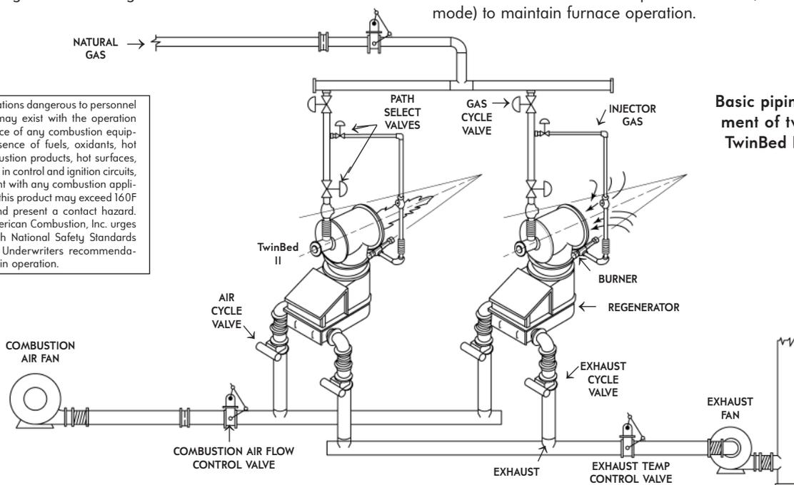
**Basic piping arrangement of two burner TwinBed II system.**
