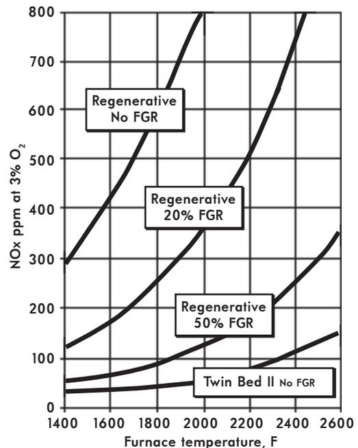
Conventional regenerative burner NO<sub>x</sub> levels vs. TwinBed II
