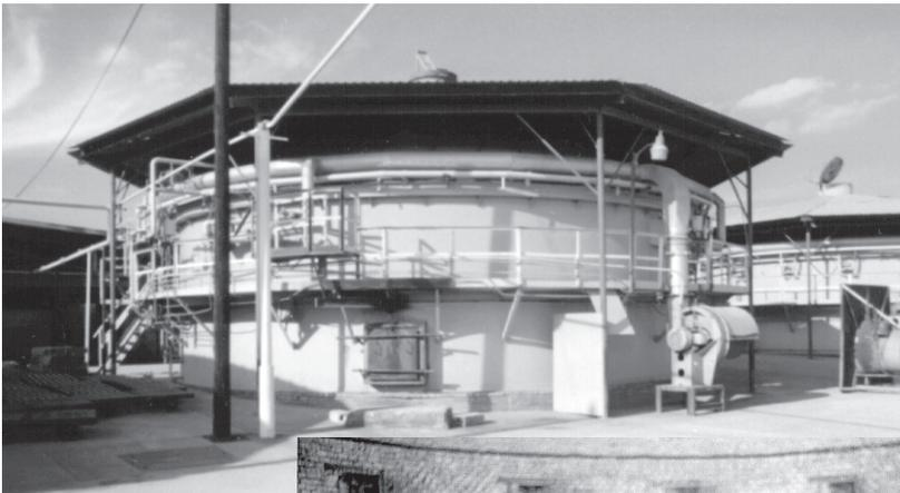
*42' diameter beehive kiln with new HiRAM<sup>®</sup> Burners and StepFire<sup>™</sup> Control System*
