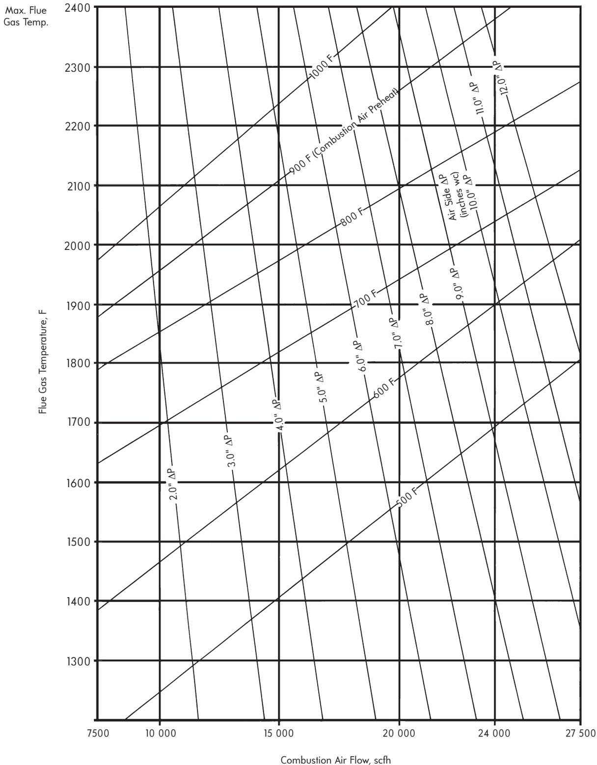
Preheats are based on typical operating conditions at 10% excess air and all flue gas flowing through recuperator.
