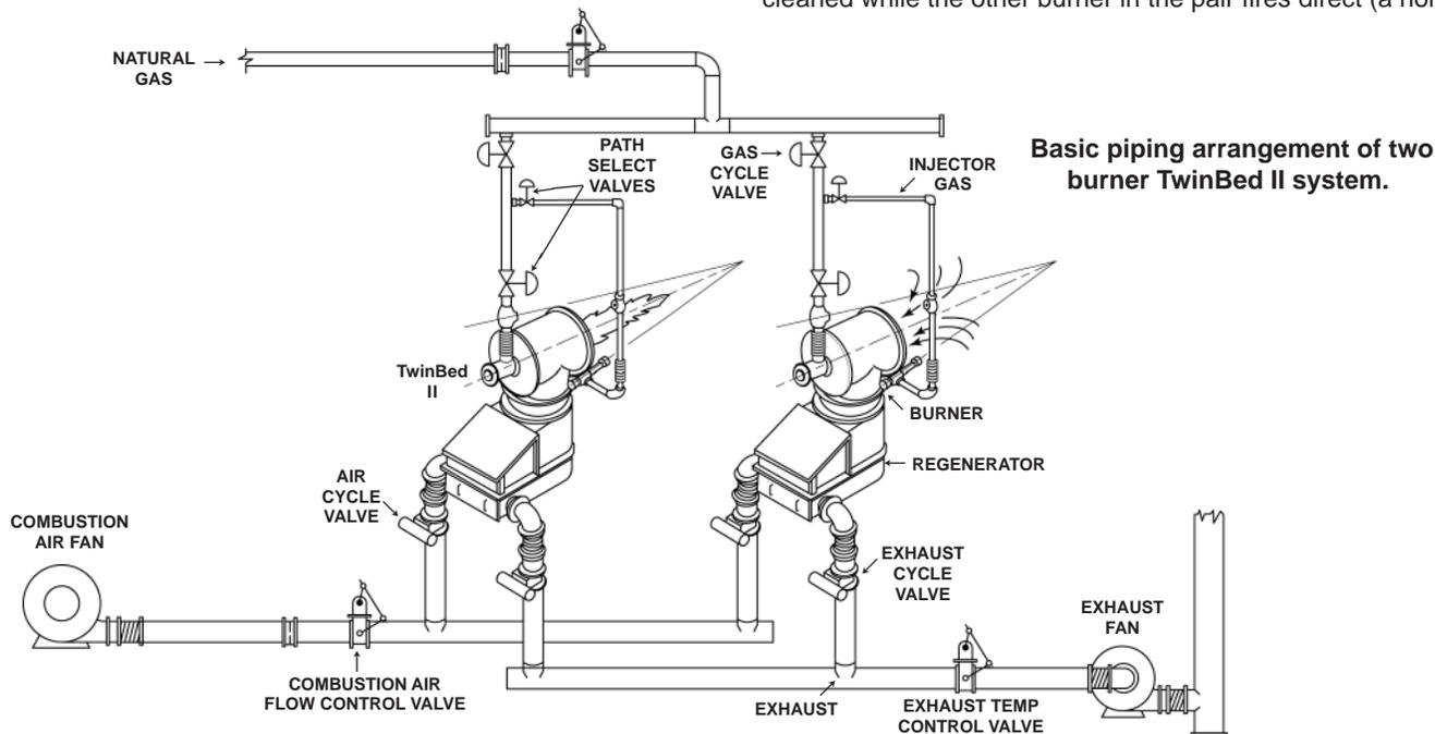
Basic piping arrangement of two burner TwinBed II system.
