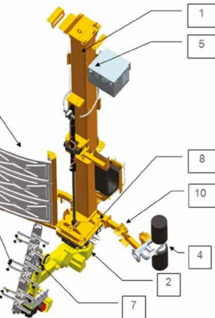
1. The modular embedded service robot is based on a 6-axis industrial robot.
