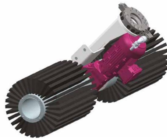
3. Rotating brush attachment to remove bath spillage.
