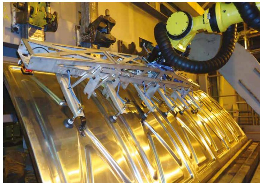
2. The ESR must be able to precisely locate, handle and replace the pot hood under operational conditions.
