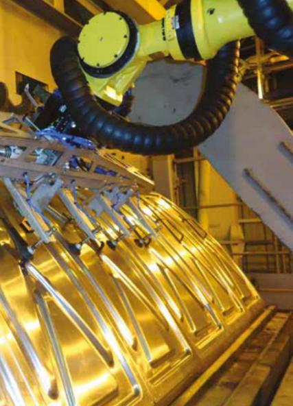
2. The ESR must be able to precisely locate, handle and replace the pot hood under operational conditions.
