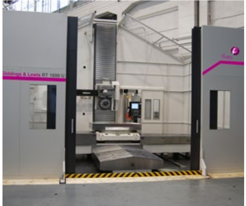
Giddings & Lewis RT 1600 U Rotary Table Horizontal Boring Mill with Integrated Contouring Head
