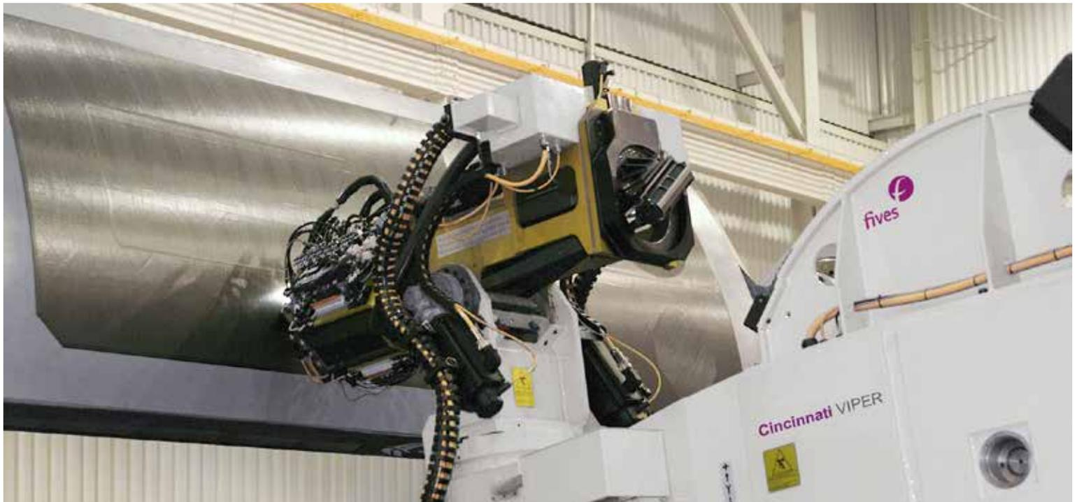
The Cincinnati VIPER fiber placement systems are the most versatile and advanced composites manufacturing equipment in production today
